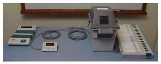
Control Unit VSDU Printer (VVPAT) Balloting Unit
